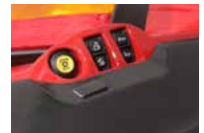
External controls are provided at the front and rear of the tractor for the hydraulic life, PTO and an additional control unit.
