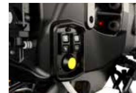
External controls are provided at the front and rear of the tractor for the hydraulic life, PTO and an additional control unit.
