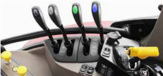
Models with purely mechanical rear remote valves also allow easy control via ergonomic levers.
