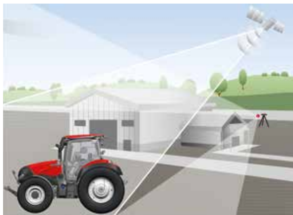
xFill bridges RTK+ signal losses of up to 20 minutes
