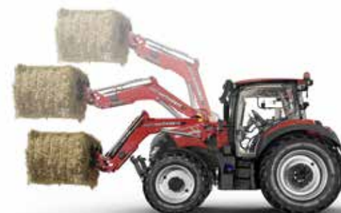
LRZ front loader with mechanical parallell guidance
