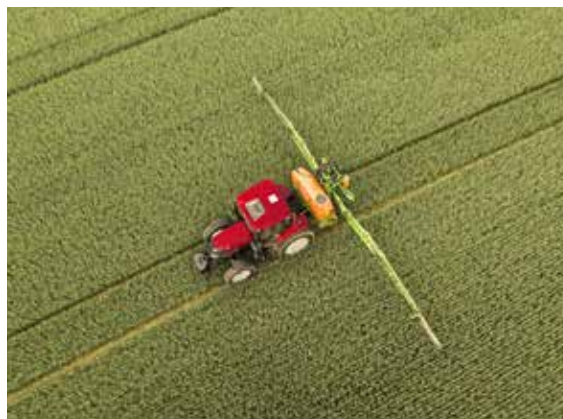
AFS AccuGuide: GPS and Glonass based track guidance
